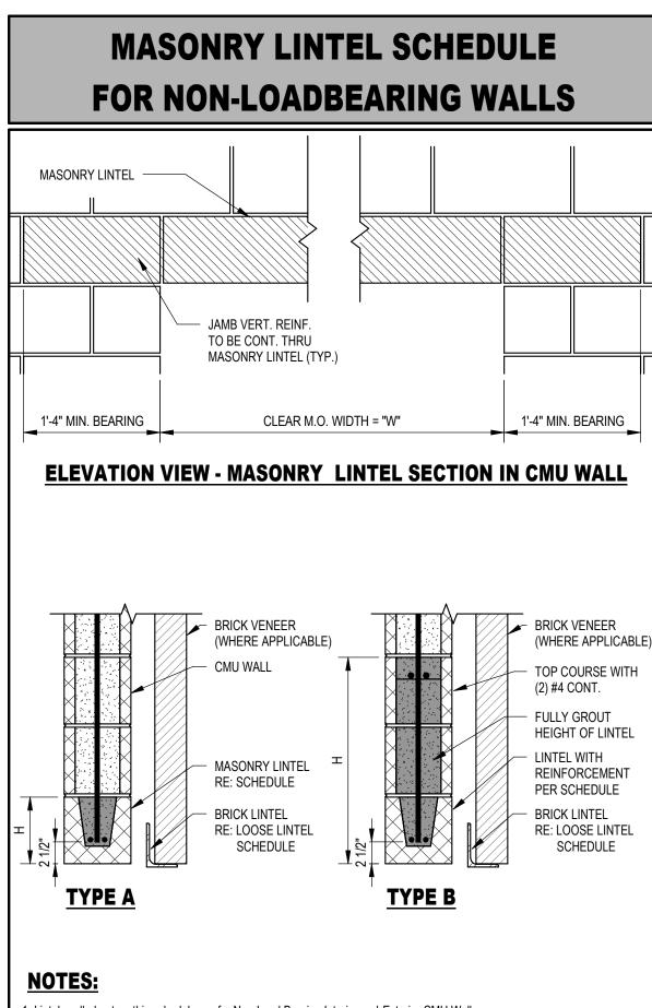
1. Lintels called out on this schedule are for Non-Load Bearing Interior and Exterior CMU Walls.
