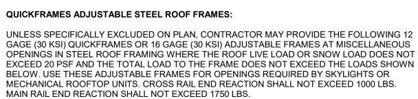
THE TOTAL FRAME LOADS SHOWN BELOW INCLUDE A 20% INCREASE FOR MECHANICAL UNITS PER IBC SECTION 1607.8.2 AND AN INDUSTRY STANDARD UNBALANCED MECHANICAL LOADING
